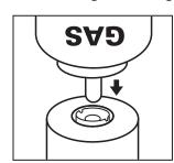
To refill the *Hammer*, turn the unit upside down and firmly push the butane can into the filling valve.
